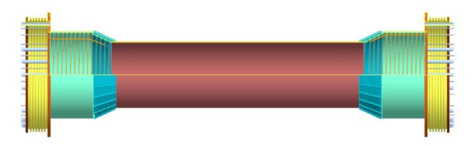
CS Casing is used as a large resistive heating element
