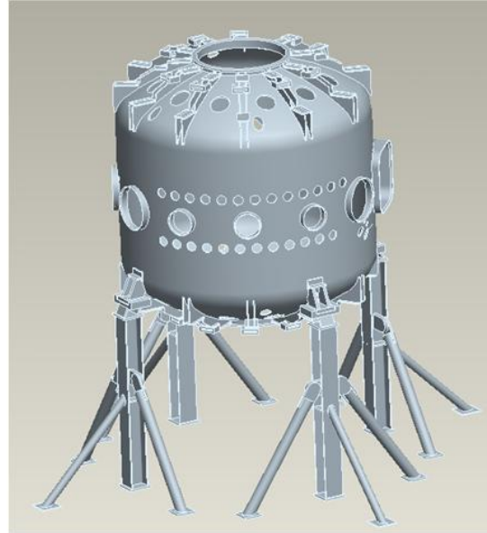
Figure 7.6.1-1 Neutral Beam Ports (left) Vessel and Supports (Right)
