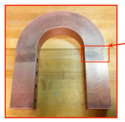
Fuji Paper pressure tests indicate >1500 psi over the entire joint surface
